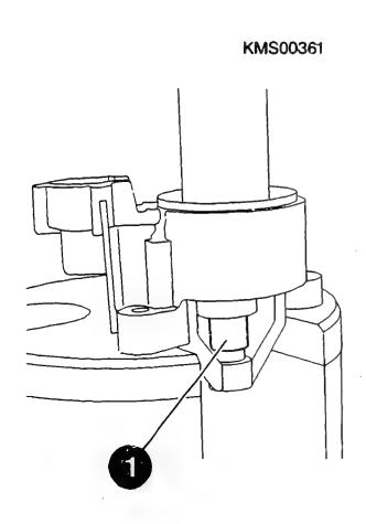
COMPONENT CHECKING AND REPAIR Checking commutator end shield Bushing of commutator end shield is always to be replaced. Removal: Use puller (1) and spring collet to pull bushing out of commutator end shield. Puller: 0 986 617 243 Spring collet diameter 10 mm: 0 986 617 250
